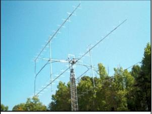
^ 2M: four M2 2mxp28 crosspolarized antennas with 21.3dbd gain. Used for eme and terrestial on a 72ft crank up layover tower. These antennas are on a computer controlled Az-El mount. Its just too distracting to work an EME station and hand control the antennas at the same time. Not impossible but a lot of work.
